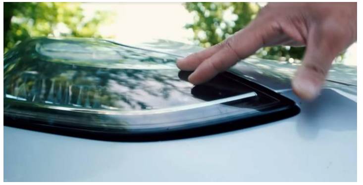
Poor Lighting Mounting/Alignment
