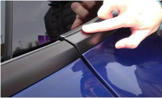
Door/Door Panel Misalignment
