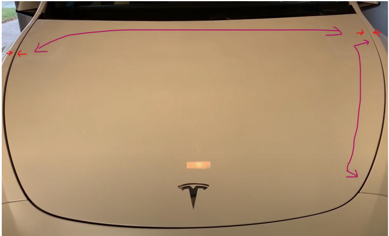
Front Trunk Panel Gap / Misalignment.
