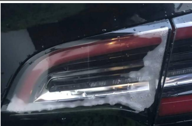
Exterior Light Condensation
