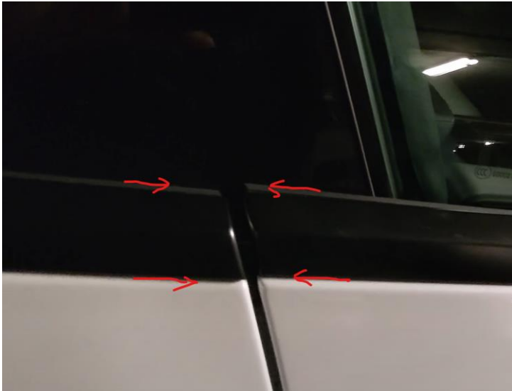
Door/Door Gap Alignment
